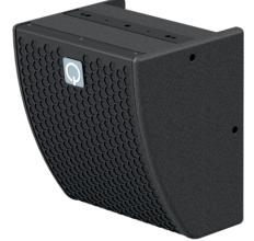
MODEL type filter power handling program power impedance sensitivity program SPL 1m peak SPL 1m frequency range dispersion weight size (wxhxd) C5 6,5"/1" coaxial 1-channel DSP control 100W 200W 8 Ohms 91dBWm 114dB 120dB 75Hz-20kHz 100° conical 3 kg / 6 lb 236 x 270 x 198 mm 9.3 x 10.6 x 7.8 inch
