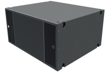
MODEL type filter power handling program power impedance sensitivity program SPL 1m peak SPL 1m frequency range dispersion weight size (wxhxd) C42 2x21" bandpass 1-channel DSP control 3600W 7200W 4 Ohms 100dBWm 139dB 145dB 38-200Hz omni 90 kg / 198 lb 1180 x 585 x 1000 mm 46.5 x 23.0 x 39.4 inch
