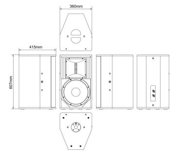
MODEL T12 5"ND AMT/12"ND full range system type filter passive power handling 800W 1600W program power impedance 8 Ohms sensitivity 97dB 1W 1m program SPL 129dB 1m 45 -20.000 Hz frequency range dispersion 80°x30° hxv, rotatable 24 kg weight 360 x 607 x 415 mm size (wxhxd)
