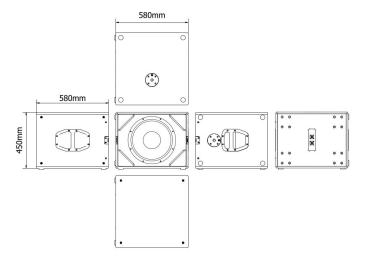
MODEL 15" bassreflex sub type filter none power handling 1300 W program power 2600 W 8 Ohms impedance sensitivity 97 dB 1W/1m program SPL 131 dB 1m peak SPL 137 dB 1m frequency range 40-400 Hz dispersion omni weight 31 kg size (wxhxd) 580 x 450 x 580 mm
