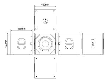
MODEL **S12** 12" bassreflex sub type filter none program power impedance sensitivity program SPĹ peak SPL frequency range dispersion weigh
