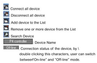
Click the icon, you will see below conversation window. Click the preferable connection mode and device model. (In this case, device model shall be "P4 controller")
