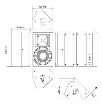
MODEL **U15** 15"/2.5" universal type full range system filter passive power handling 800W program power 1600W 8 Ohms impedance sensitivity 98 dB/W/m program SPL 130 dB peak SPL 136 dB frequency range 45 -19 kHz dispersion 60°x50° hxv rotatable weight 23 kg size (wxhxd' 435 x 735 x 410 mm
